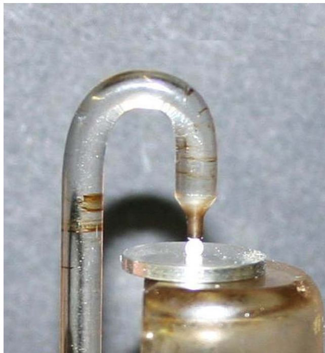
Fig. 2. TMA sample holder designed for measuring the T_g of a film on a pellet (in situ).
